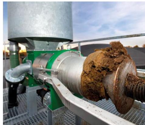
Figura 3 – Prensa parafuso (*screw press*)
